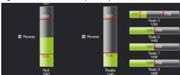
Fig4: Calibration of directions using RC controller
