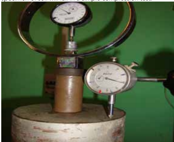
Fig 3. Soil sample placed in compression device
