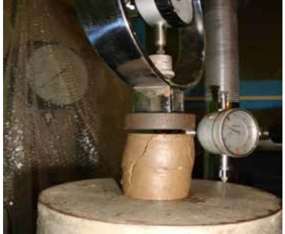
Fig 4. Soil sample failure
