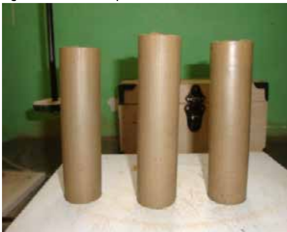
Fig 2 Samples for unconfined compression test (b) Testing
