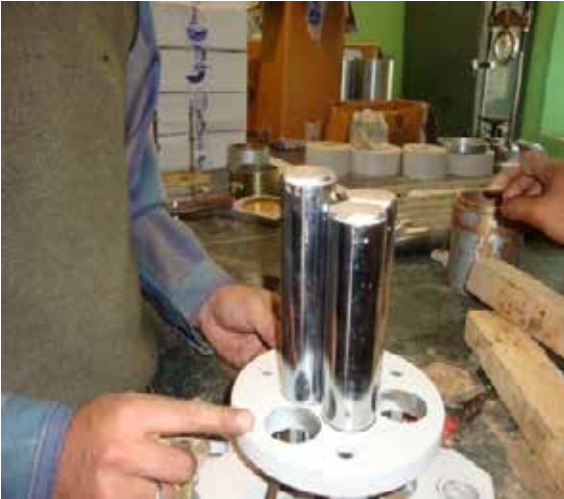
Fig 1: Soil in tube sampler
