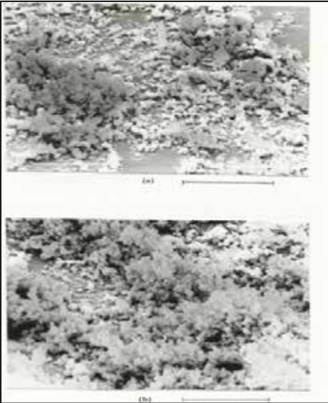
Figure 8.18: SEM micrographs of the particle morphologies of zirconia powders, showing the loosely packed particles of (a) Y-PSZ (U) and (b) Y-PSZ (M). Original magnification. 2500 (Scale bar = 10µm).
