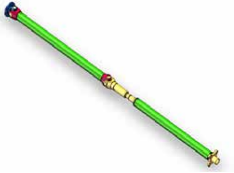
Figure 1. The cardanic transmission assembly modeled with Solidworks (general view)
