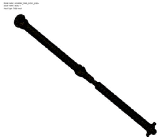
Figure 2. The meshed cardanic transmission model (general view)
