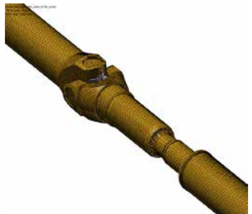
Figure 3. The meshed cardanic transmission model (detail)
