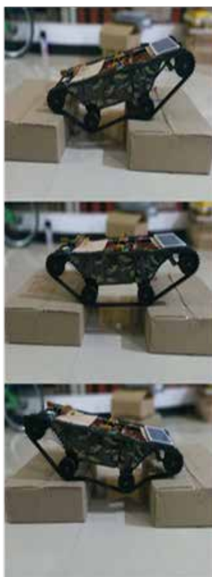
Figure 8: Shows the robot crossing a gap. (Clockwise)
