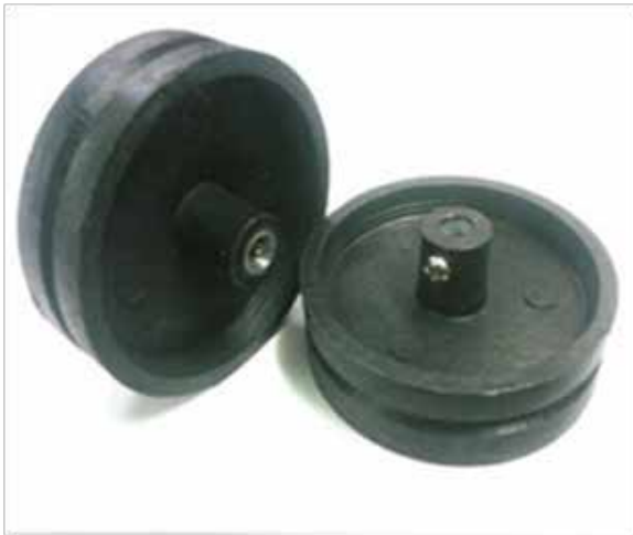
Figure 3: The grouser belt and wheel used in the model • The vehicle has 8 wheels among which 4 wheels are driven by high torque motors, two wheels are driven by low torque motors and 2 wheels are idle. All the wheels are moved in a synchronized manner using a gripper belt, among the 4 wheels which are connected to high torque motors 2 wheels are at front top position and the remaining 2 are at rear bottom, the 2 wheels which are connected to low torque motors are at rear bottom position as shown in the figure. Each wheel has a circumferential v-groove which helps in the meshing of belt with wheel and avoids slipping of belt. The wheels are mounted coaxially with the motor shafts and dead axle to prevent whirling. Corresponding wheels on left and right portion of the vehicle are coplanar. Two gripper belts are used to move the wheels synchronously; the belts are made from rubber and have external grousers. V groove helps to mesh the belt with wheels.
