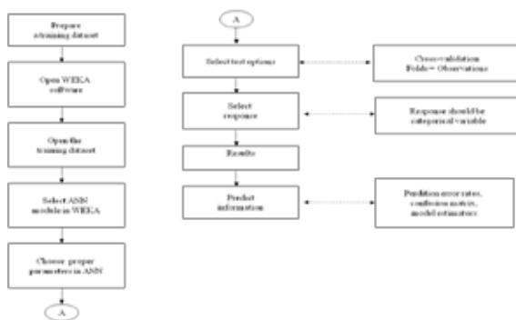
Fig.6: Flowchart showing steps involved in constructing an ANN classifier model under WEKA environment to predict hepatitis occurrences.
