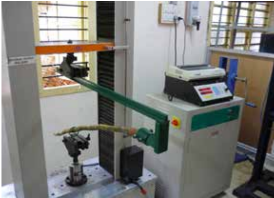
Figure 1. Experimental set up for measuring bending resistance
