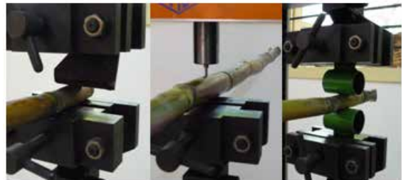
Figure 2. Experimental set up for measuring cutting, penetration and crushing resistance
