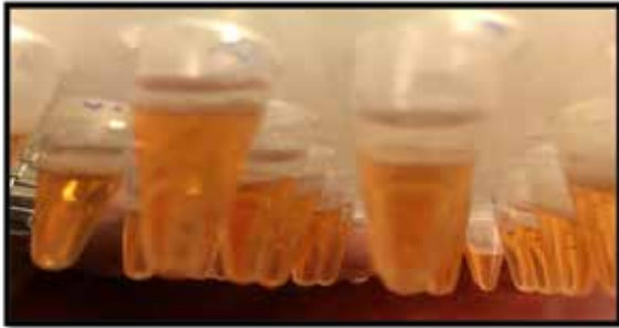
Figure 2 : Shows eppendorf tube contained three phase : aqueous phase ,intermediate phase and organic phase , in the chloroform – phenol method
