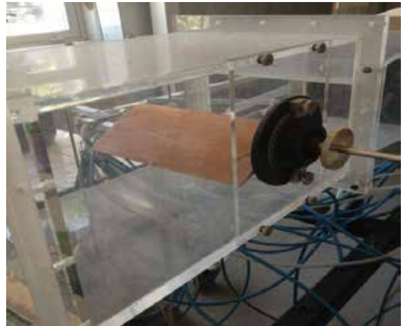
Fig 3- Experimental set up of wind tunnel [4]
