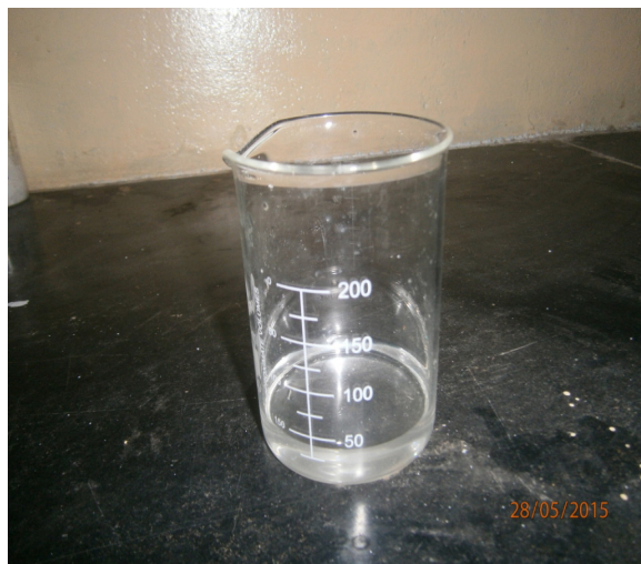
Figure 2. Clear aqueous solution of fuel and oxidizer mixture in solution combustion synthesis used.
