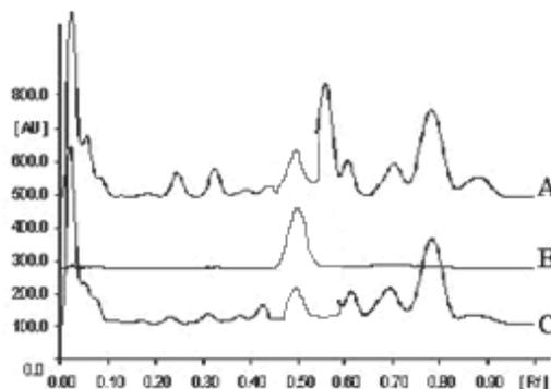
**Figure 7. HPTLC-densitogram at 530 nm of *O. Tenuiflorum* with Beta Sitosterol standard after derivatization with anisaldehyde-sulfuric acid reagent: (A) Sample Solution 1 (Akola), (B) oleanolic acid standard; (C) Sample Solution 2 (Mumbai)**
