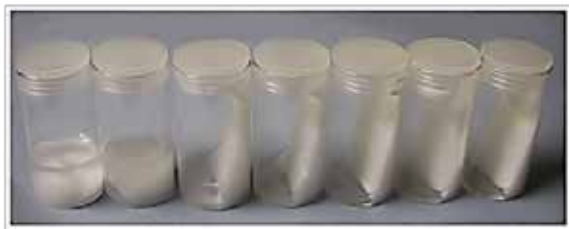
Fig. 1 Effect of the duration of exposure to the UV lamp on the formation of the poly (BuMA-co-EDMA) monolith.
