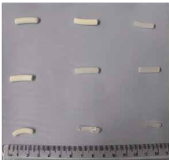
Fig.2 The appearance of the poly (BuMA-co-EDMA) monoliths prepared using different porogenic solvent systems before washing them with methanol.
