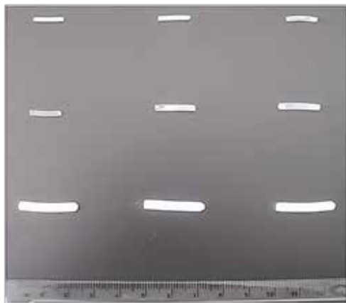
Fig.3 The appearance of the poly (BuMA-co-EDMA) monoliths prepared using different porogenic solvent systems after washing them with methanol to remove the unreacted monomeric materials using Soxhlet extraction with methanol at 80 °C for 24 hours. 3.3. Characterisation of the fabricated materials
