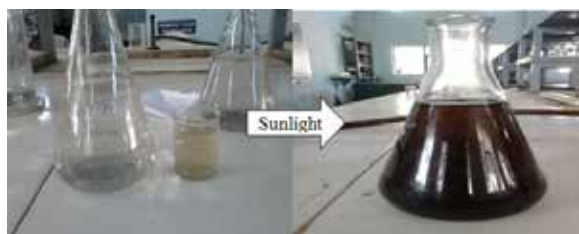
Fig.2 (a) Caralluma fimbriata plant extract (b) \text{AgNO}_3 mixed with Caralluma fimbriata plant extract.
