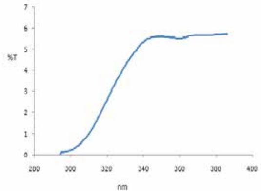
**Fig 2 UV transmittance spectra of uncoated coir fiber**
