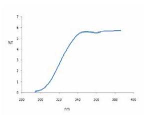
Fig 2 UV transmittance spectra of uncoated coir fiber
