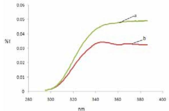
**Fig 3 UV transmittance spectra of a) Ag coated (10 min) b) Ag coated (20min)**
