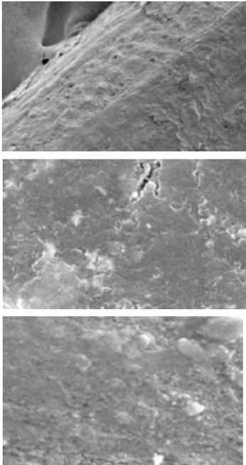
**Fig 1 SEM images of a) uncoated coir fiber b) Ag coated (10min) c) Ag coated (20min)**
