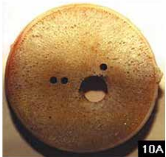
Helical blade: impaction causes bone compaction
