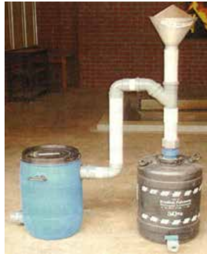
Figure 2: Photograph of Developed Composite Rain Water Harvesting Unit.
