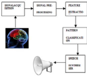
Fig. 1 Block diagram of Brain computer interface
