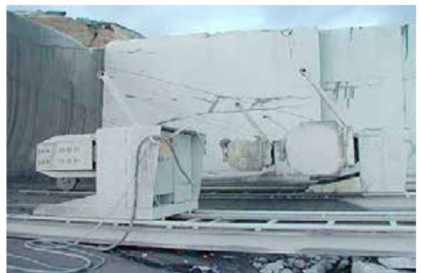
Photo 2: Use of diamond wire saw for marble block recovery
