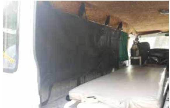
Fig 2: Resin Sheets in Ambulance
