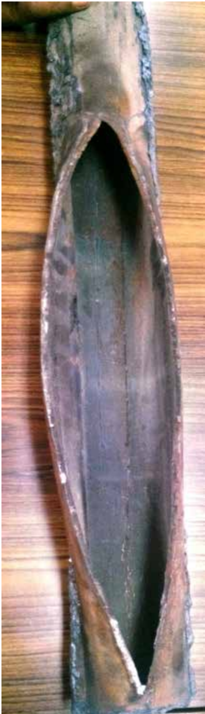
Fig. 2 : Failure of Platen Super Heater Tube
