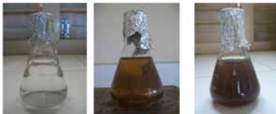
Figure.1 Aqueous solution of AgNO 3 before and after addition of leaf extract of Ocimum sanctum .
