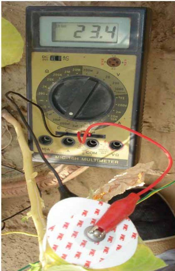
Figure 3: The leaf capacitance measurements using ECG electrode
