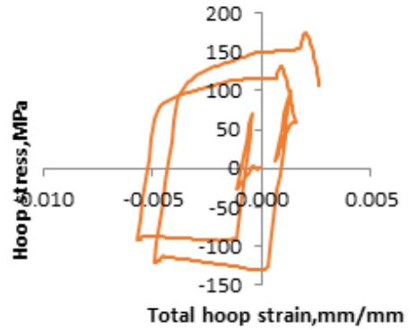
Fig11: variation of stress with total strain MISO+CHAB Model
