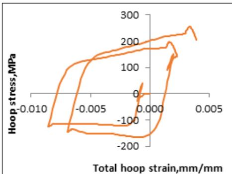
Fig9 Variation of stress with total strain MKIN model
