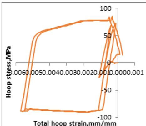
Fig10 Variation of stress with total strain Thermal Loads And Pressure Loads For Section Near
