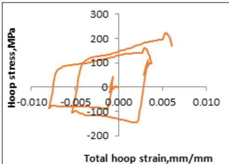
Fig8 variation of stress with total strain MISO+CHAB Model
