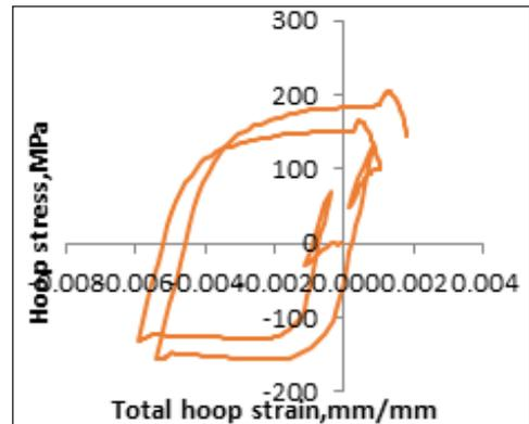
Fig 12 : variation of stress with total strain
