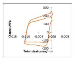
Fig6 Variation of stress with total strain Thermal Loads and Pressure Loads For Section Near Throat MKIN Model
