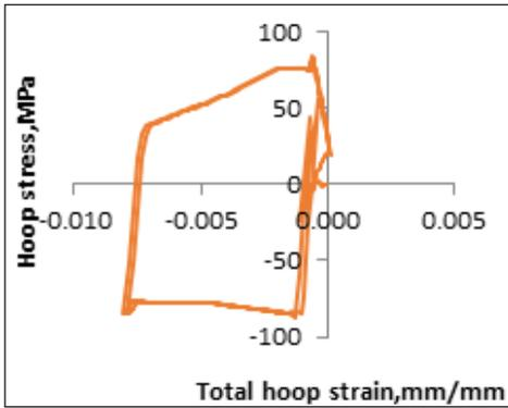
Fig7 variation of stress with total strain MISO Model
