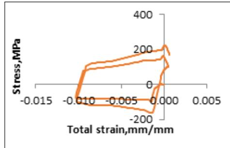
Fig 5 Variation of stress with total strain MISO+CHAB Model
