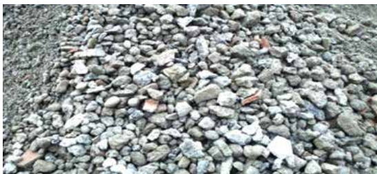
Fig. 3 Crushed demolished cement concrete waste
