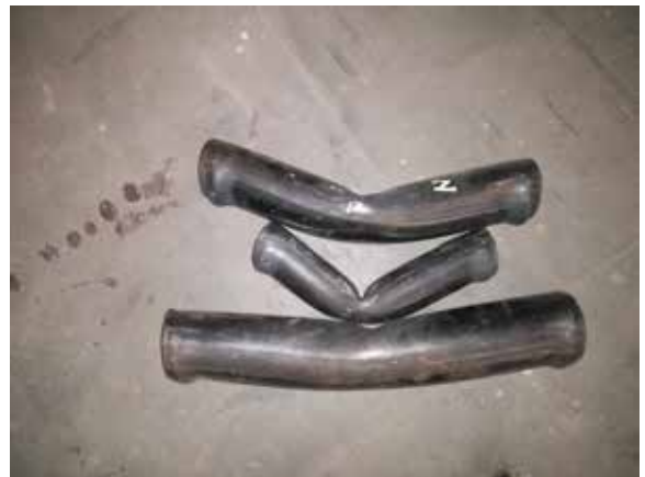
Fig.2 hollow steel tubes at failure
