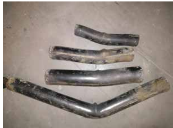
Fig.3 SCC infilled steel tubes at failure
