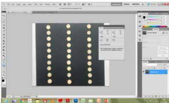
Fig 2 Software analysis of samples to evaluate CIELAB values
