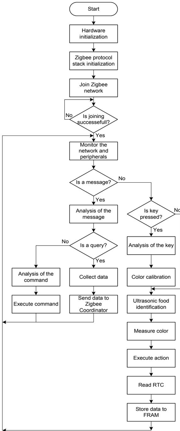
Figure 5: Terminal node program flow chart
