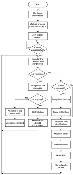
Figure 5: Terminal node program flow chart
