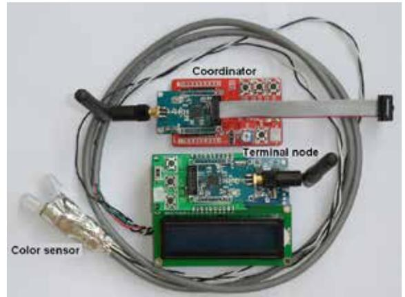
Figure 6: Prototype microprocessor system
