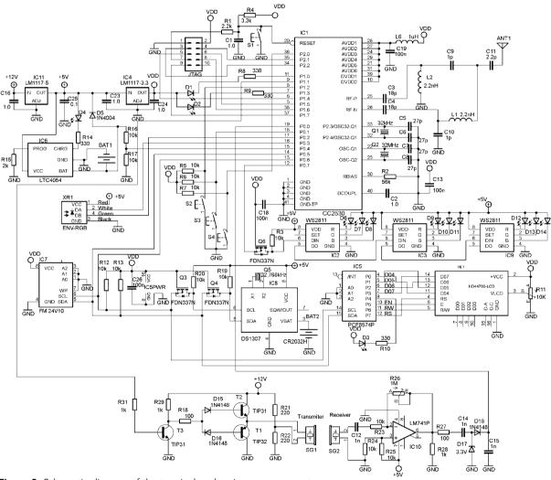
Figure 3: Schematic diagram of the terminal node microprocessor system
