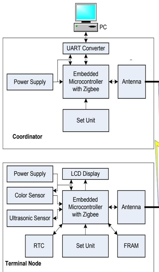
Figure 1: Block diagram of the system
