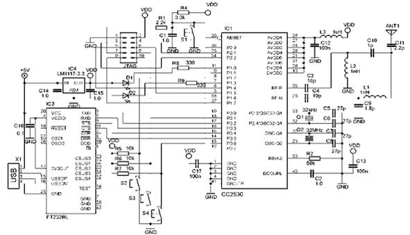
**Figure 2:** Schematic diagram of the coordinator microprocessor system
