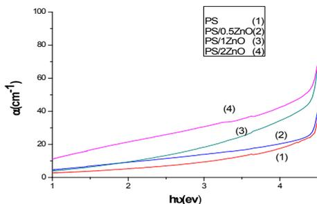
Figure (6). Variation of the absorbance coefficient against wavelength
