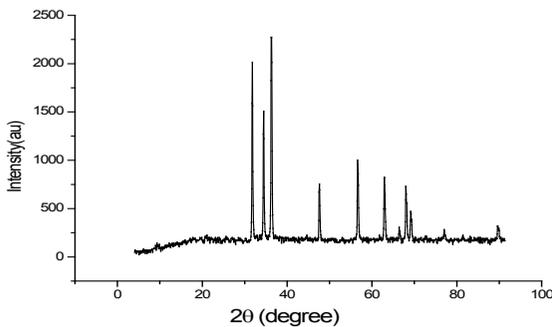
**Figure (1).** XRD pattern of ZnO nanoparticle.
