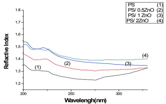
Figure (7). Variation of the reflective index against wavelength
