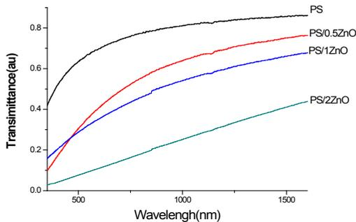
Figure (5). Variation of the transmittance against wavelength
