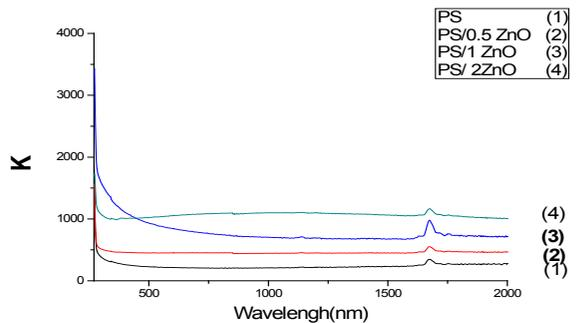
Figure (8). Variation of extinction coefficient against wavelength
