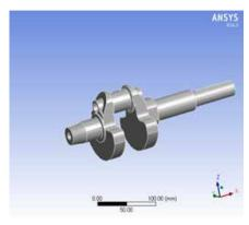
Fig 1: 3-D model of Crankshaft using Pro-E
