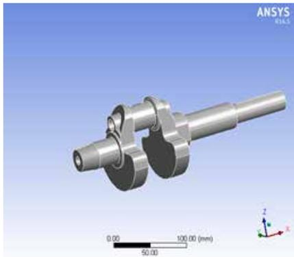
Fig 1: 3-D model of Crankshaft using Pro-E
