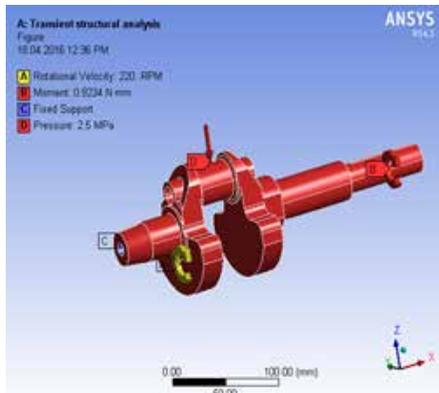
Fig 2: Input Values Applied On The Crank Shaft
