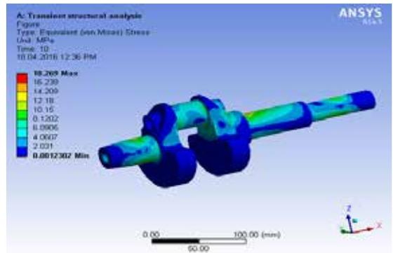
Fig 4: Structural Analysis of crank shaft (Equivalent Stress)
