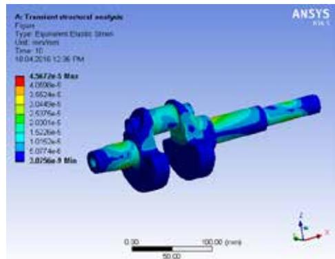
Fig 5: Fatigue Analysis of crank shaft (Equivalent Elastic Strain)
