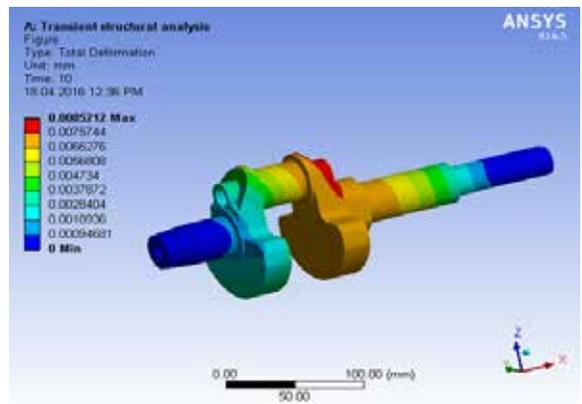
Fig 3: Structural Analysis of crank shaft (Total Deformation)
