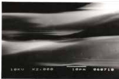
Figure 6: SEM image of untreated polyester fabric
