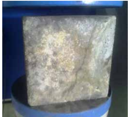
Fig.6 Test Specimen at Cracking
