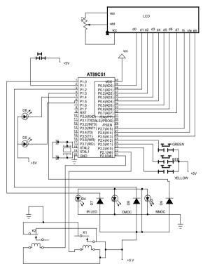
In this circuit AT89S51 get the signal from Bar sensor, MOC7811, switch control, IR Sensor.
