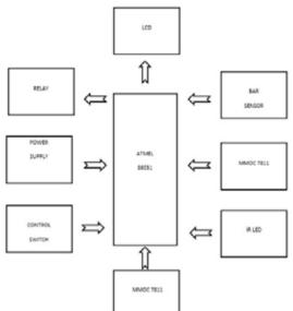
The Atmel AT89S51 is an 8051 based Full Static CMOS controller with Three-Level Program Memory Lock, 32 I/O lines, 2 Timers/Counters, 6 Interrupts Sources, Watchdog Timer, 2 DPTRs 4K Flash, 128 Bytes On-chip RAM.
