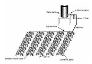
Source: (RCSD 2008) Schematic design of a low-cost Drip irrigation system.
