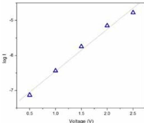
**Figure-2:** Plot of log I vs. V for AZO photoelectrode. **Figure 4** shows the J-V measurements for a PEC cell under the UV illumination. FF and η was calculated by using equations (2) and (3), respectively.
