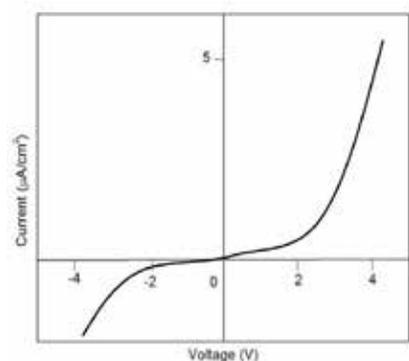
**Figure-1:** I-V characteristics of AZO photoelectrode (in dark).
