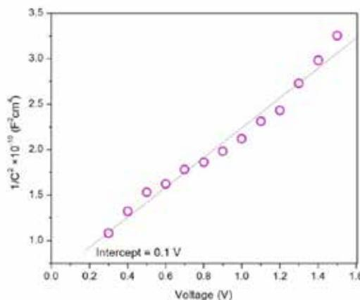
**Figure-3:** C-V characteristics of AZO photoelectrode.
