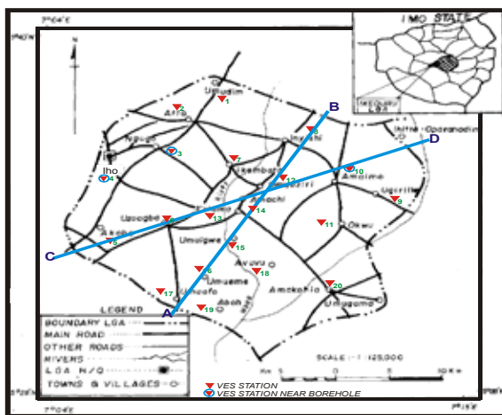
Fig. 1 Map of the Study Area showing the VES Stations and Interpretative Geoelectric Cross Section (IGCS) Traverse.
