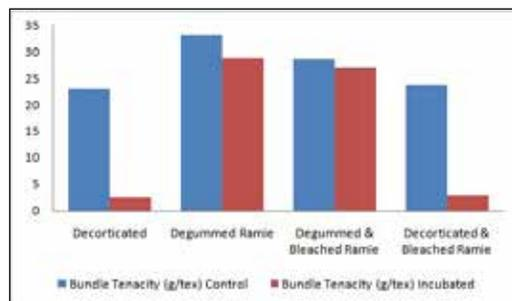
**Fig.3: Bundle Strength of Ramie fibre before and after soil burial test**
