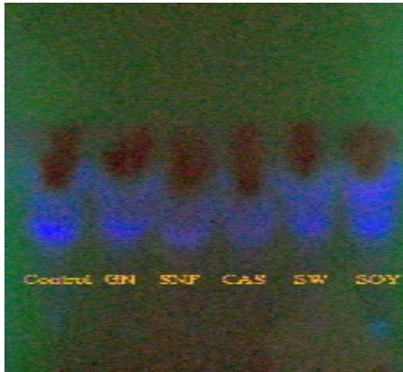
Fig 1.2 TLC plate showing presence of AFB 1 of selected isolates with standard AFB 1 (control) under UV light (365 nm).
