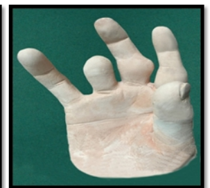
Fig 3: Master Model poured with type III dental stone
