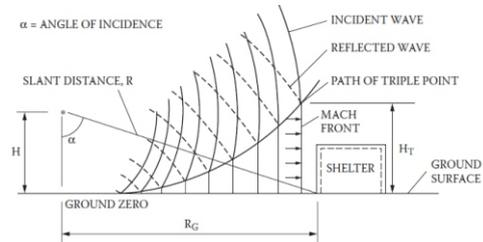
Figure 3: Crash environment from air burst
