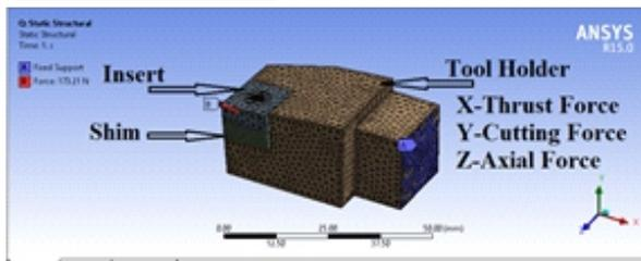
Figure (1): Meshing and boundary condition of tool holder
