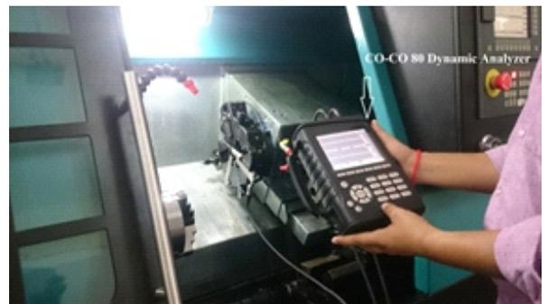
Figure (3): CNC Machine and Dynamic Analyzer
