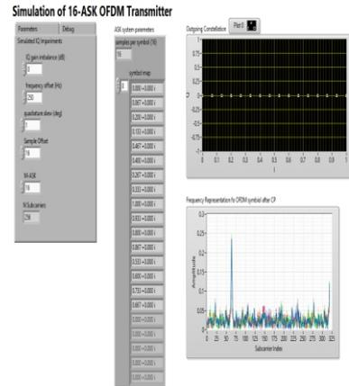
**Fig. 6 Simulation of 16- ASK OFDM Transmitter**
