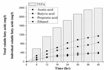
Figure 6: Changes VFAs with time (*Enterococcus faecalis*)
