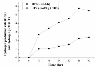
Figure 5: Hydrogen yield and production rate with time (*Enterococcus faecalis*)
