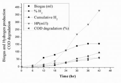
Figure 1: Biogas, Hydrogen production, COD degradation with time (*Bacillus subtilis*)
