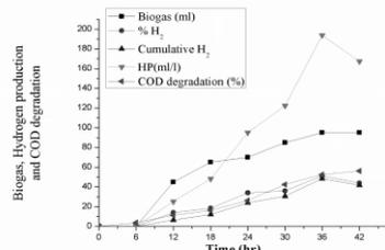
Figure 7: Biogas, Hydrogen production, COD degradation with time (*Acinetobacter calcoaceticus*)
