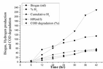
Figure 4: Biogas, Hydrogen production, COD degradation with time (*Enterococcus faecalis*)
