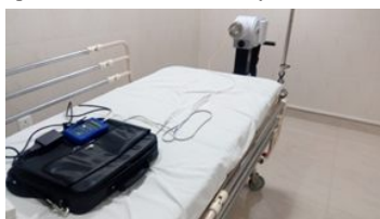
Figure 1: Calibration of MOSFET dosimeter in Ir-192 source
