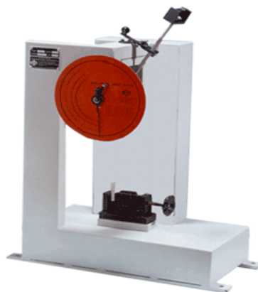
Fig.1 Experimental setup for impact strength test
