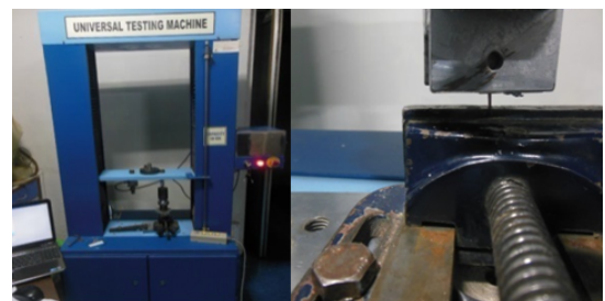
Fig.2 The tensile strength of all Gutta-percha cones after disinfection was measured using computer controlled universal testing machine
