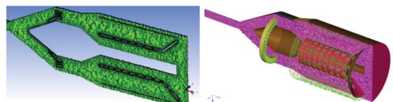
**Fig -4 Volume Tetra Mesh - Cut Sectional View along the flow**
