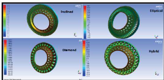
**Fig -7 Static Pressure Variations over the Swirler with guider**
