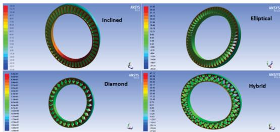
**Fig -6 Static Pressure Variations over the Swirler Configurations**
