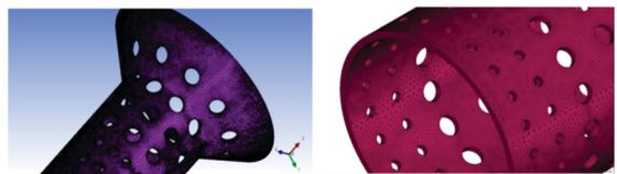
**Fig -3 Inner and Outer Annulus of the Micro Gas Turbine Engine**
