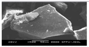
This SEM image provided further insight into the morphology and size of the produced nanoparticles. It is evident from the figure that the biosynthesized silver nanoparticles are in different size and shapes and mostly observed as individual particles as well as a few aggregates.
