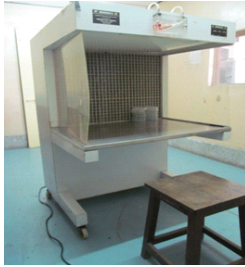
Figure 1 Laminar air flow Instrument to maintain sterile working environment [3]
