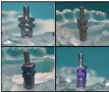
Fig 2: (a) Non-modified coping b) Sandblasted coping (c) Adhesive coated coping d) Sandblasted & adhesive coated coping
