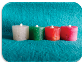
Figure 3. Composite Resin Build-Up of 3mm Diameter and 3mm Height
